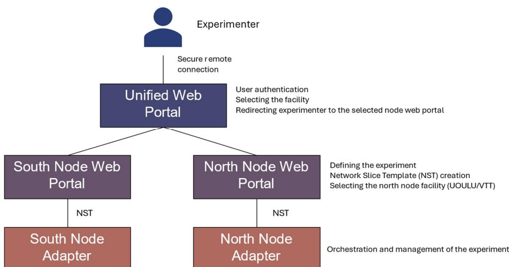
Figure 16. 6G-XR trial controller architecture with example workflow for the 6G-XR North Node.
