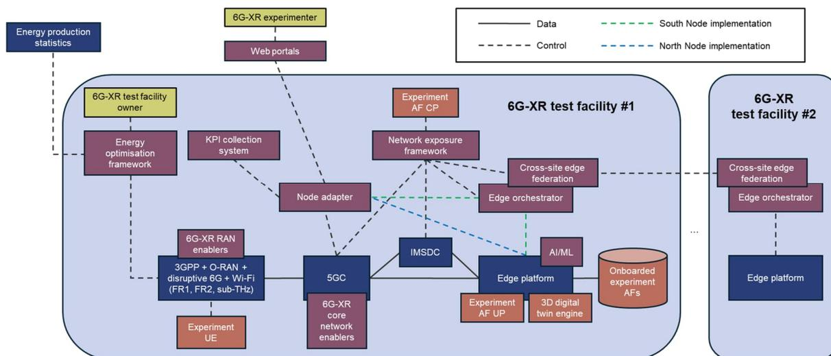
Figure 2. 6G-XR reference architecture – Interconnected view.
