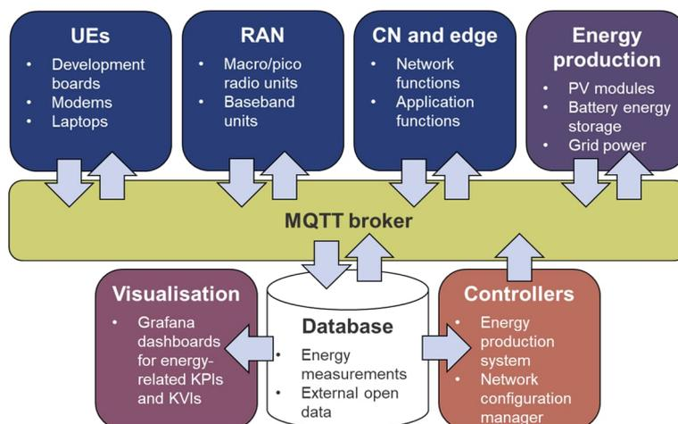
Figure 8. Main components of the energy measurement framework.
