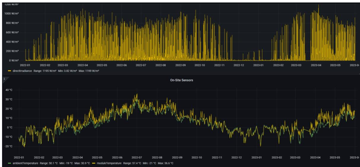
Figure 7: On-site sensor data collected over two last years (solar irradiance at top and temperature at bottom)
